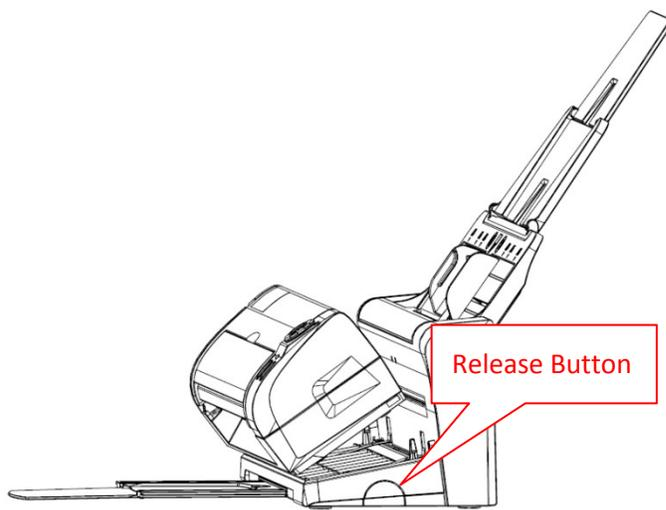
After you have removed the external tape, press the **release** button on the **right**-hand side to undock the scanner. Lift the Scan Module up and forward to undock it. Remove the protective foam from between the Scan Module and the Dock.
