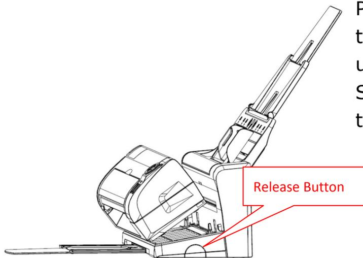
Press the **release** button on the **right**-hand side to undock the scanner. Lift the Scan Module up and forward to undock it.
