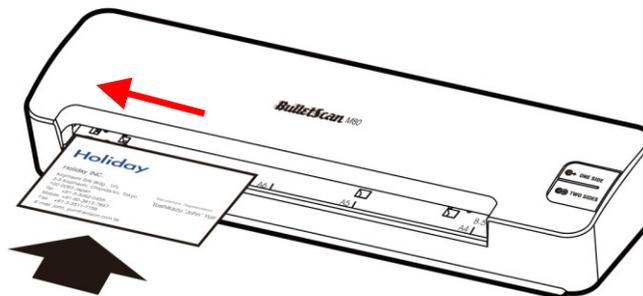
2. Align the original to the left side of the paper feed slot.
